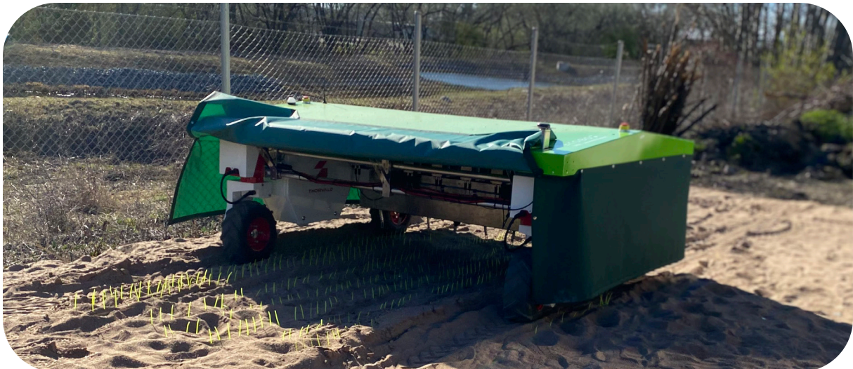
Ekobot WEAI – autonomous weeder
